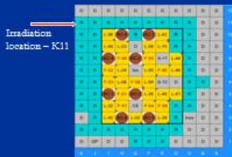
Fig. 3. TRIGA SSR 14 MW present core configuration
