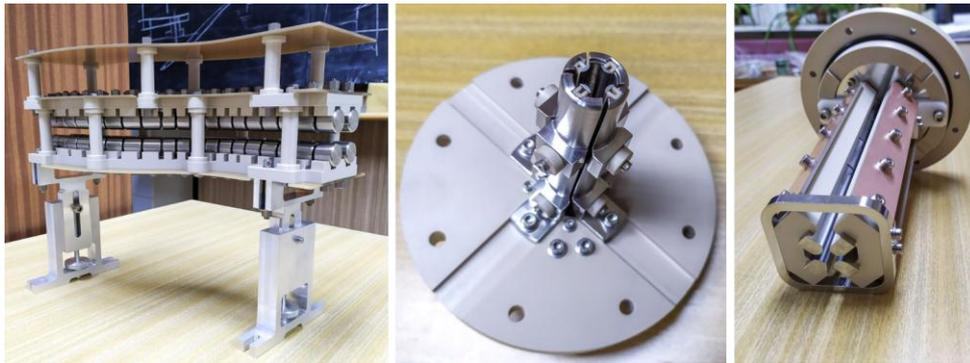
**Fig. 5.** The SRFQ, microRFQ and LRFQ parts of the GALS ion guide system.
