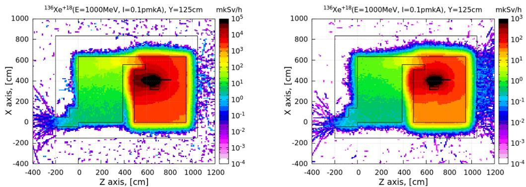
**Figure 3.** FLUKA simulations of radiation conditions in the GALS setup physical cabin. Left-hand side: neutron radiation, right-hand side: photon radiation.
