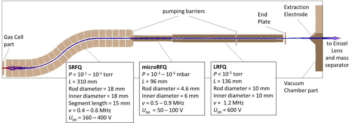
**Figure 4.** The ion guide model within GALS front-end vacuum chamber.
